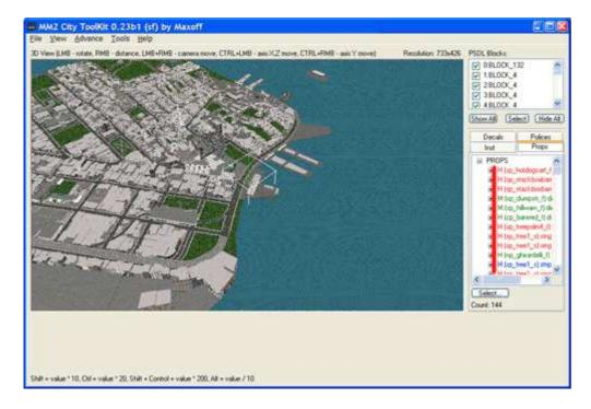
Props view is colored. Green means directed props, red means single props and blue means strips. Please check pathset file specification for details.
