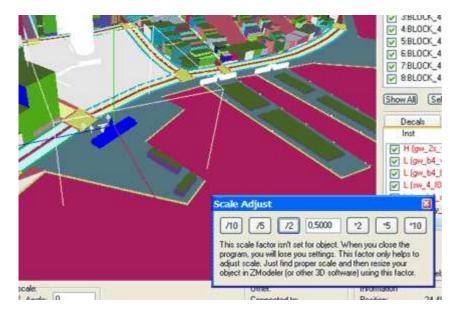
The scale factor isn't set for object. When you close the program, you will lose you settings. This factor only helps to adjust scale. Just find proper scale and then resize your object in ZModeler (or other 3D software) using this factor.
